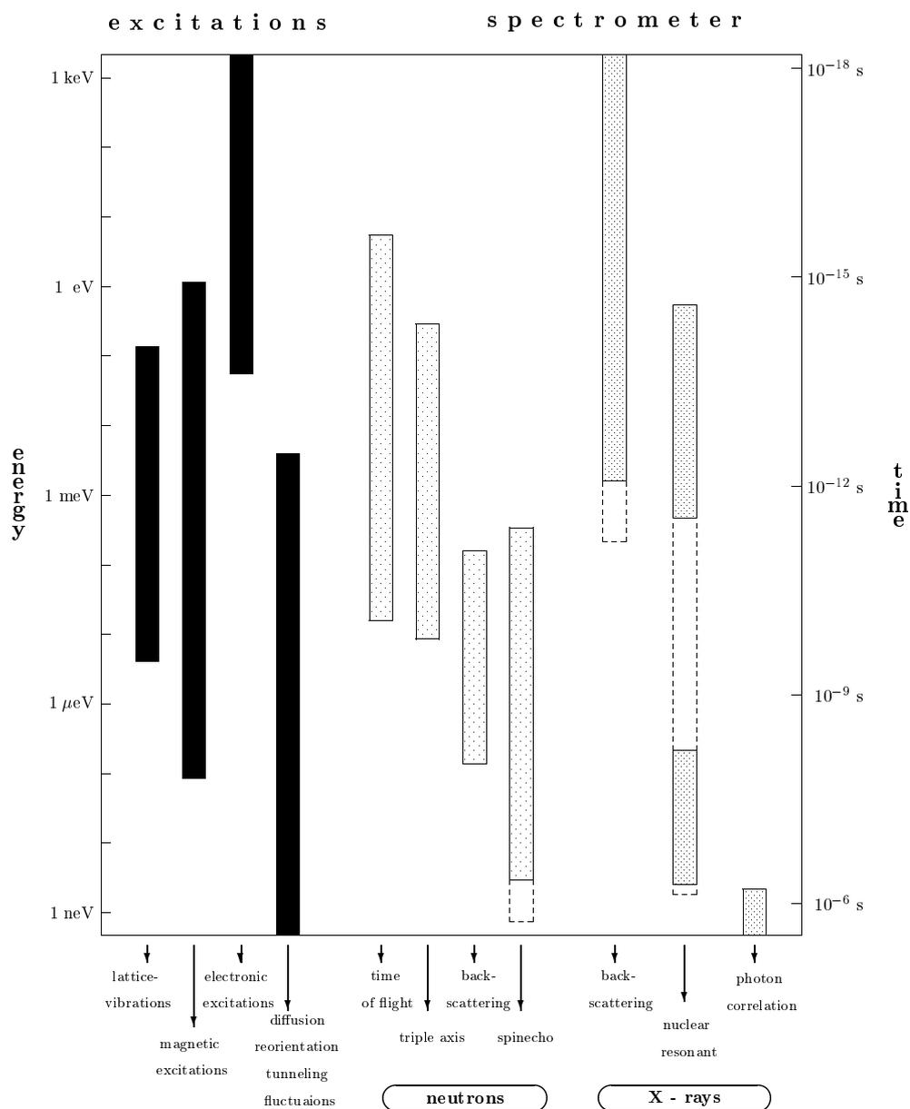
**Figure 1.** Excitations with their typical energy and time scales and the appropriate spectrometer for the detection with x-rays and neutrons.
